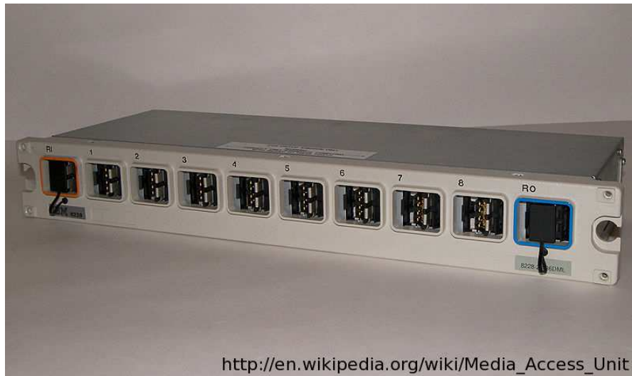
Figura B.8. MAU: Media Access Unit
